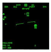
In this mode, rather than displaying a god's-eye view from above, the radar display is a 60-degree cone from center to edge, looking forward. Radar returns appear right or left of the center of the display proportionate to their actual position to the right or left of the nose of your aircraft. Their position between the top and bottom of the display indicates their distance from you, depending on the radar range.
