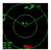
The Easy display consists of two concentric circles with a pie wedge. The circles are range rings and the pie wedge is the view your radar sees in front of you (the radar cone). You are located in the center of that circle and the view is a god's-eye view looking down.
